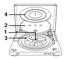
**1** Move the metallic parts inside the larger gear in the direction of arrows.
